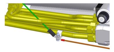
With the Pro Control controls, the grounding connection is integrated in the wiring harness and is an important component of the system's automatic supervision. This line is needed, for example, to identify short circuits or cable breaks in the system and to deactivate specific functions in the case of any faults.
